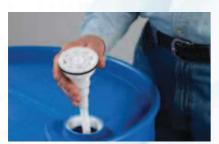
Place the drum insert assembly in drum.
