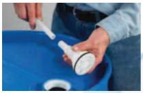
Fully press dip-tube into drum insert
