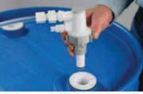
Insert coupler into drum insert assembly.
